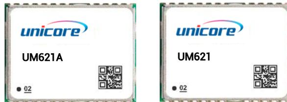
Figure 1-1 UM621 Series Modules (Left: Automotive; Right: Industrial)
